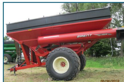
**Brent 1080 Grain Cart**, tarp, scales, 35.5L-32 tires, 20" discharge auger
