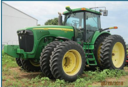
**2005 JD 8320 MFA Tractor**, 14.9-34 front duals, front suspension, 18.4-46 rear duals, HID lights, quad hydraulics, active seat, Green Star ready, 3-pt., big 1000 PTO, 8 front wts. & 2-1500# rear wts., 3,200 hrs., SN RW8320P035030
