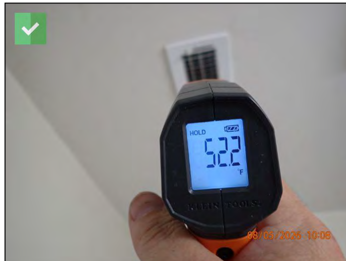
A/C Differential 23.2 Degrees F
