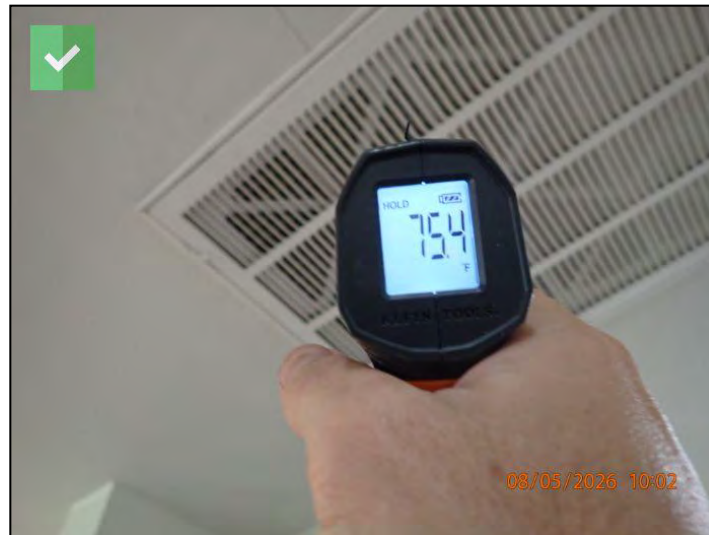
A/C Differential 23.2 Degrees F
