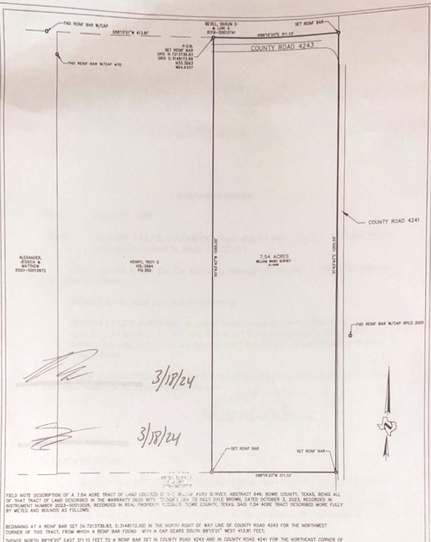
THENCE NORTH 8876'20" EAST 311.10 FEET TO A REINF BAR SET IN COUNTY ROAD 4243 AND IN COUNTY ROAD 4241 FOR THE NORTHEAST CORNER OF THIS TRACT;
