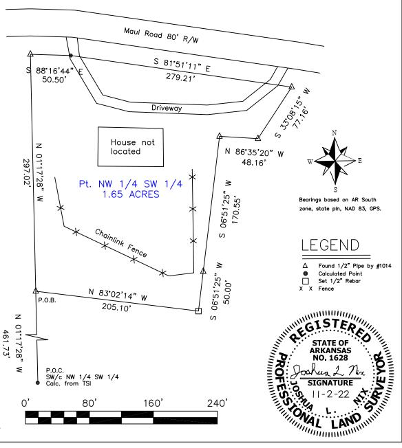
I certify that this survey drawing was done by me or under my supervision and was based on an actual ground survey on November 2, 2022. Iron monuments were found or set as shown on this drawing. This survey is correct to the best of my knowledge. This survey is subject to visible and invisible easements, setbacks, and right of ways, shown or otherwise. This is a boundary survey only, utilities not shown.
