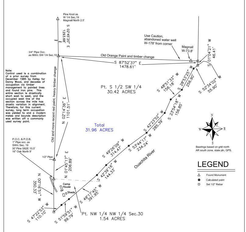
I certify that this survey drawing was done by me or under my supervision and was based on an actual ground survey on February 22, 2024. Iron monuments were found or set as shown on this drawing. This survey is correct to the best of my knowledge. This survey is subject to visible and invisible easements, setbacks, and right of ways, shown or otherwise. This is a boundary survey only, utilities not shown.
