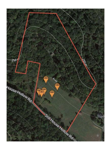
**SURVEYOR NOTE**: Grid stakes should extend at least 50 feet beyond the area(s) marked in the image(s) above. If, at the time of grid staking, the area(s) needs to be mowed, bush hogged, forestry mulched, or otherwise maintained please inform the customer immediately.
