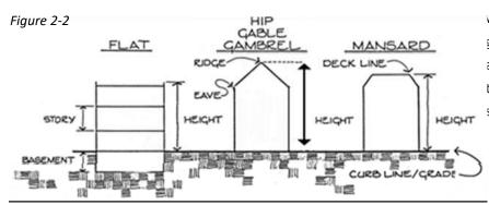
Height, Structure - The vertical distance from the grade of the finished surface adjacent to the structure to the highest point of the structure or any attachment.
