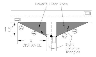
Step 1. On your scaled site plan, show your driveway or street intersection through the street. Indicate a point center of your driveway or street located 15 feet back from the edge of the curb line, edge of the pavement, or edge of travel way.
