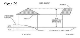
**Grade** – The average elevation of the finished grade at the center of all walls of a building (See figure 2-1)
