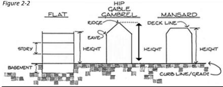
Height, Structure - The vertical distance from the grade of the finished surface adjacent to the structure to the highest point of the structure or any attachment.
