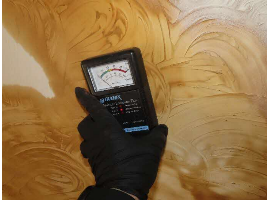
Photograph 17: A comparative moisture reading on the stain.
