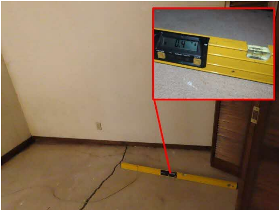
Photograph 12: A slope reading on the east side of the crack.
