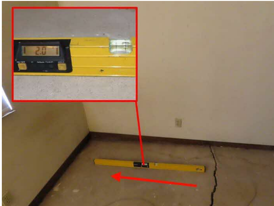
Photograph 13: A slope reading on the west side of the crack.
