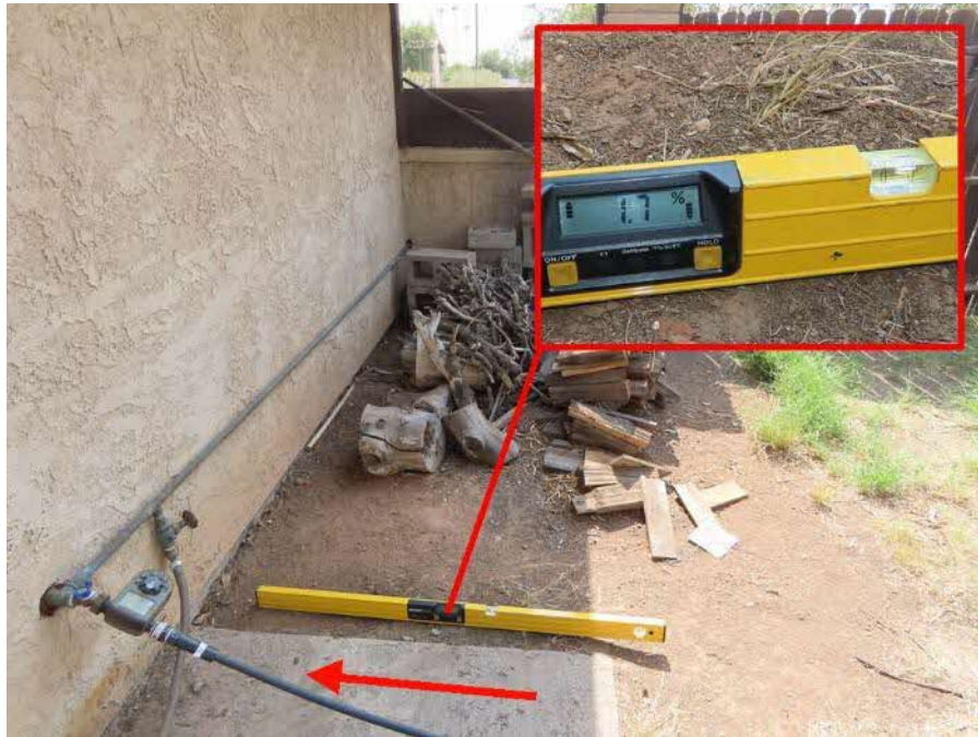
Photograph 21: A grade slope reading near the west end of the north side.
