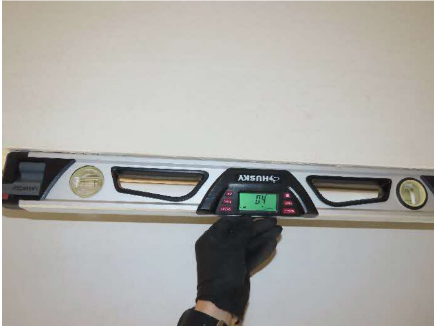
Photograph 15: A slope reading at the top of the window on the west wall.
