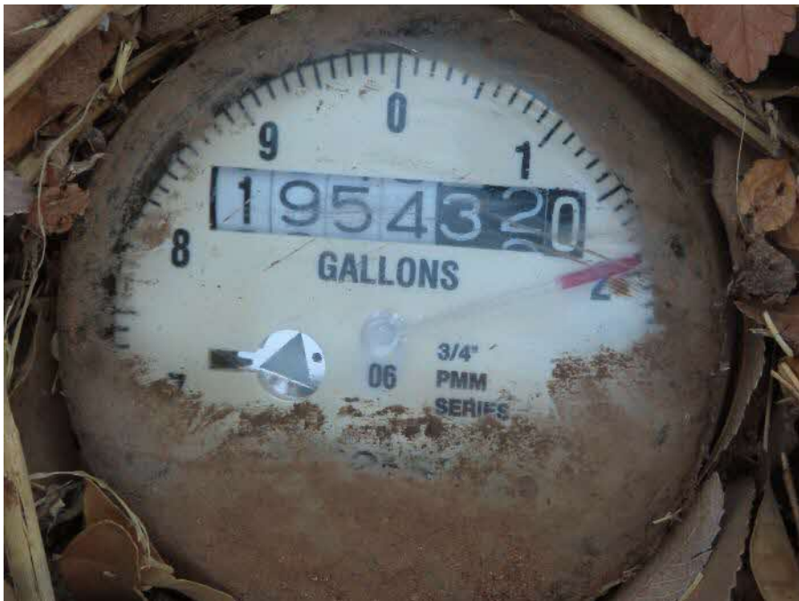
Photograph 24: The water meter at the beginning of the leak test.
