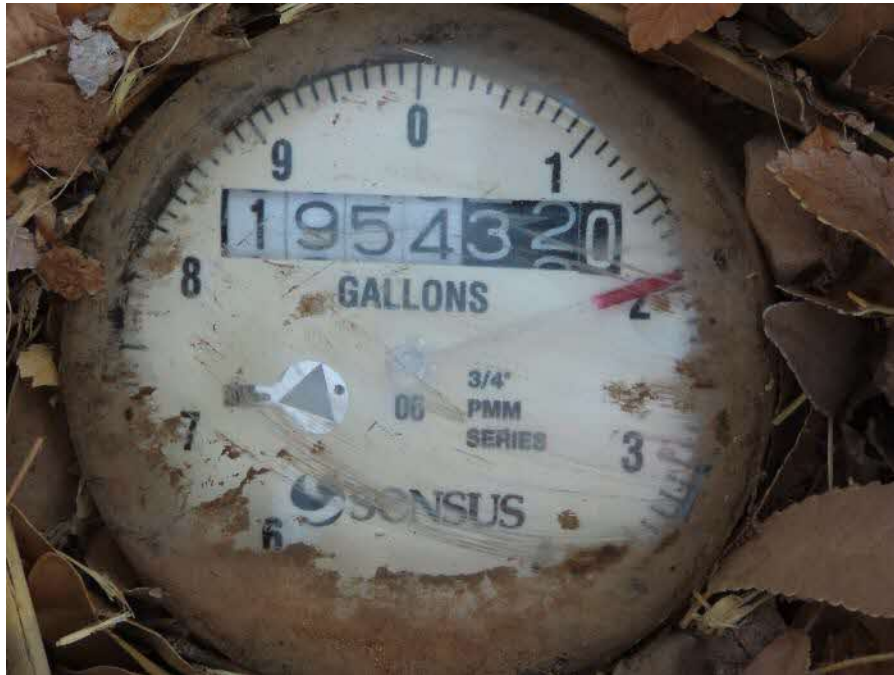
Photograph 25: The water meter at the end of the 28 minute leak test.
