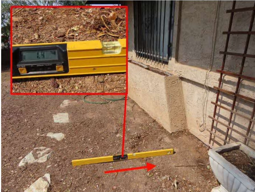
Photograph 19: A grade slope reading near the north end of the west side.
