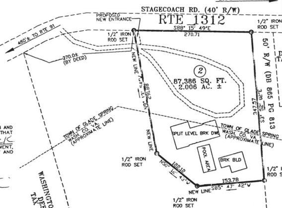
THERE IS HEREBY RESERVED A 20' WIDE DRAINAGE AND UTILITY EASEMENT ALONG ALL LOT LINES. 10' ADJACENT TO ALL INTERIOR LOT LINES AND 20' CONTIGUOUS TO ALL OUTSIDE BOUNDARY LINES. THIS IS IN ADDITION TO ANY DRAINAGE AND UTILITY EASEMENTS SHOWN HEREON
