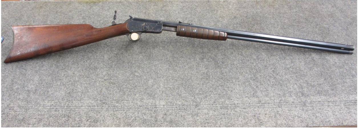
Marlin 20-A .22 Long Rifle, pump action, Octagon Barrel, Original Marble's tang sight, mfg 1907-1922
